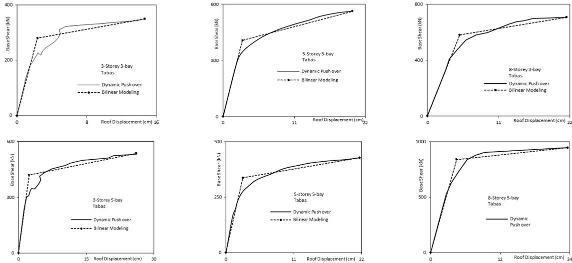
Fig. 6. Equivalent bilinear elasto-plastic model for dynamic pushover curve.
