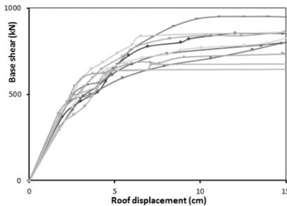
Fig. 5. Dynamic pushover curves for 5 stories five-spans structure.
