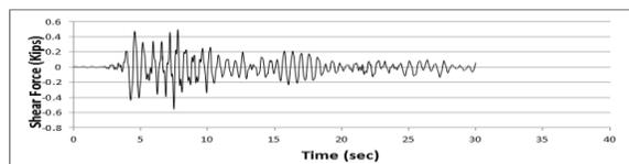
**Fig. 2. b.** Shear response time history for exterior column of the first floor (IDARC).
