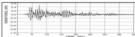
**Fig. 2. a.** Shear response time history for exterior column of the first floor (Laboratory [37]).
