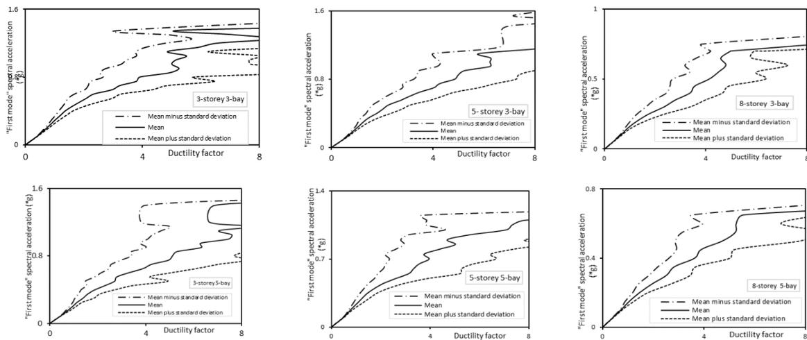
**Fig. 4.** IDA curves of structures.
