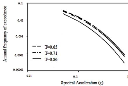
Fig. 7. Seismic hazard curves (Yazdani et al., 2015).
