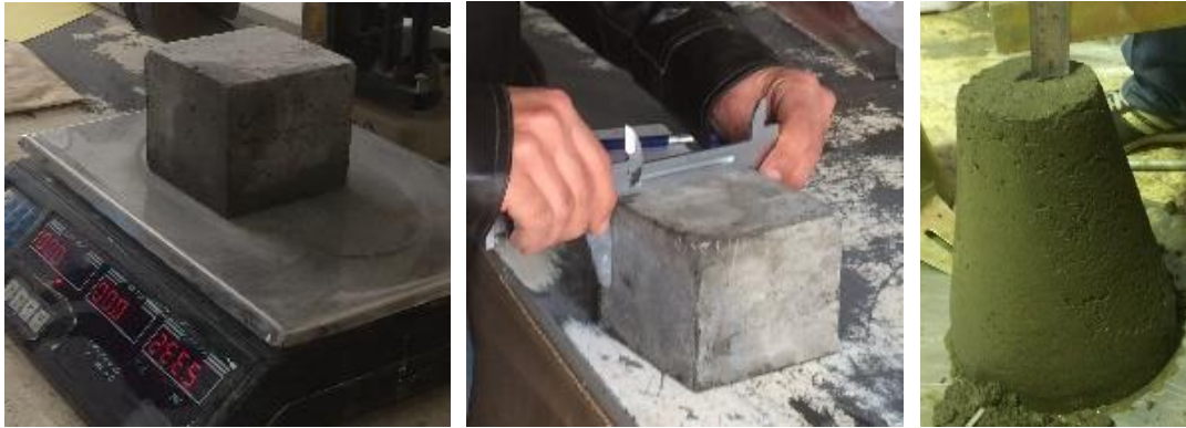
Fig. 9. Preparing and testing concrete specimens.
