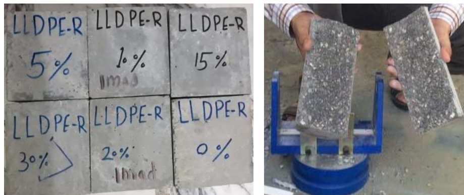
Fig. 8. Tensile strength of LLDPE-R concrete for specimens containing SF and without SF.
