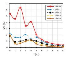
Fig 7. The effect of dynamic load frequency on the foundation settlement ratio ( $G = 5000 \ kPa$ ,  $Q_0 = 50 \ kN$ ).
