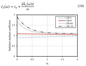
Fig 6. Dynamic damping coefficient curve [15].
