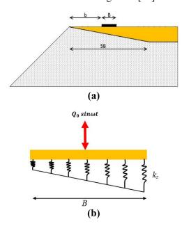
Fig 5. Changes in stiffness and damping (a) from the slope edge and (b) beneath the foundation.
