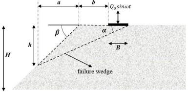
Fig 2. The plane sliding level considered below the foundation.
