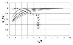
**Fig 4.** Changes in the stiffness ratio of the foundation adjacent to the slope to the foundation located on the flat ground [14].
