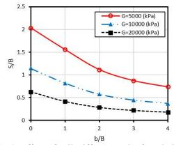
**Fig 8.** Effect of soil stiffness on the foundation settlement ratio.
