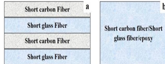
Fig.1. Schematic diagram of, (a) Laminated (multi-layer hybrid composite) and (b) single-layer hybrid composite
