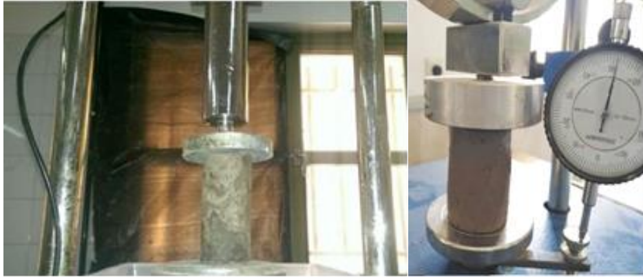
Fig 6. The prepared grout sample to be placed under the loading device and an overburden of 0.5 kg.
