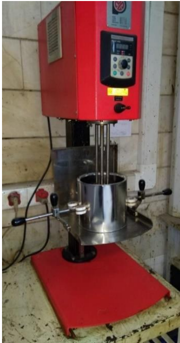
Fig 1. The high shear mixer apparatus.
