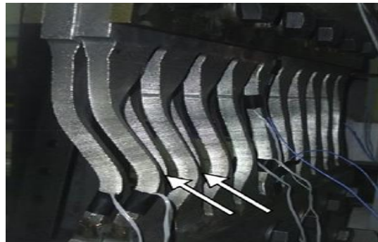
c. buckling of the damper legs model examined by Lee et al. [28].
