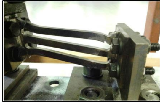
b. buckling of the damper legs model examined by Tagawa et al. [27].
