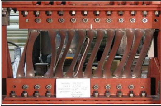
a. buckling of the damper legs model examined by Ma et al. [26].
