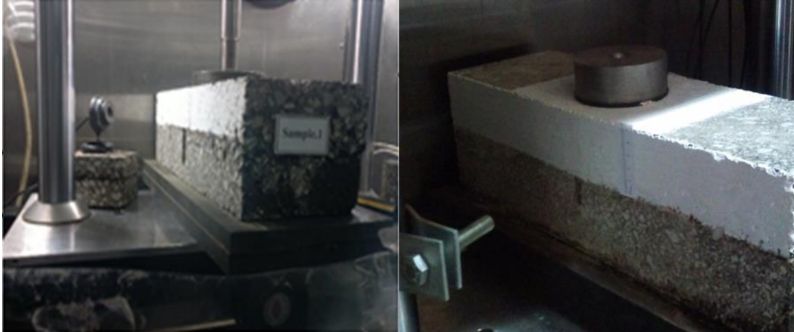
Fig. 3. The UTM225 test device used for testing.
