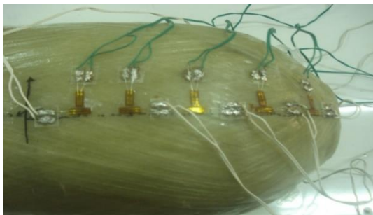
Fig. 13. Fully filament-wound composite pressure vessels
