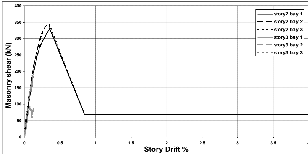
Fig. 13. Masonry infill shear versus story drift for 3 story frame model 3-O with 17 cm thickness - designed frame+strut.
