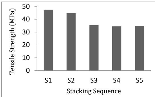
Fig. 21. Variation in specimen tensile strength with regard to stacking sequence
