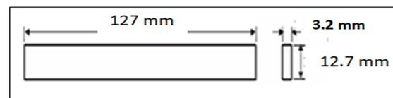
**Fig. 10.** Flexural test specimen dimensions
