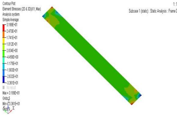
Fig. 31. Maximum stress in XY for the S4 Sample
