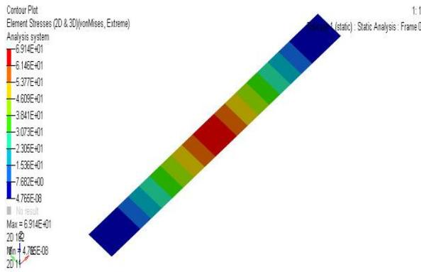
Fig. 45. Maximum von Mises stress for the S3 Sample.
