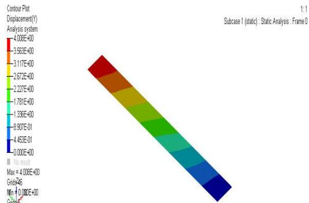
Fig. 30. Maximum displacement in the Y direction for the S3 sample
