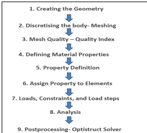
Fig. 11. General procedure of modeling and analysis in Hypermesh
