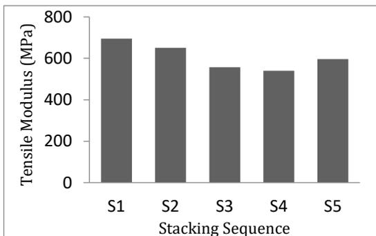
Fig. 22. Variation of tensile modulus of specimens with respect to stacking sequence
