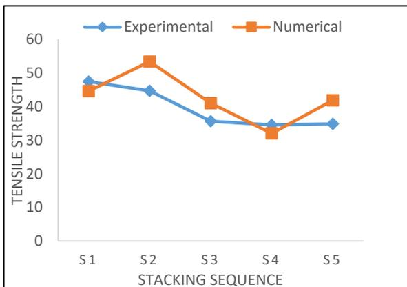
Fig. 36. Comparative study of tensile strength results with respect to stacking sequences.
