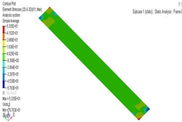
Fig. 27. Maximum stress in XY for the S2 Sample
