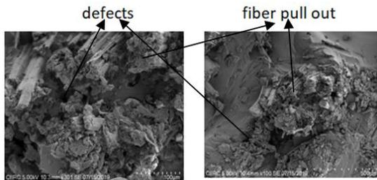
Fig. 39. Tensile test fractured SEM images of S2 specimen (15% B and 15% J)
