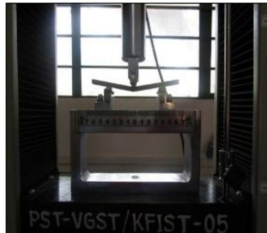
**Fig. 9.** Computerized Flexural Testing Machine setup
