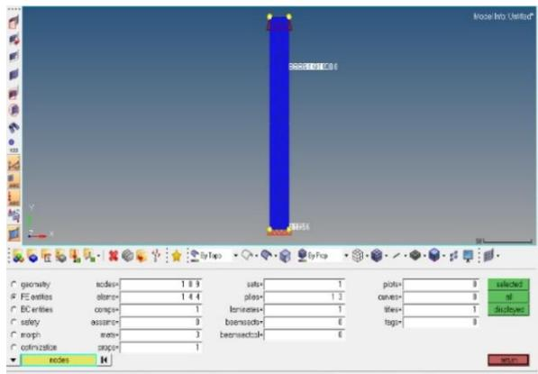
Fig. 13. Discretization process: number of elements: 144, number of nodes: 189
