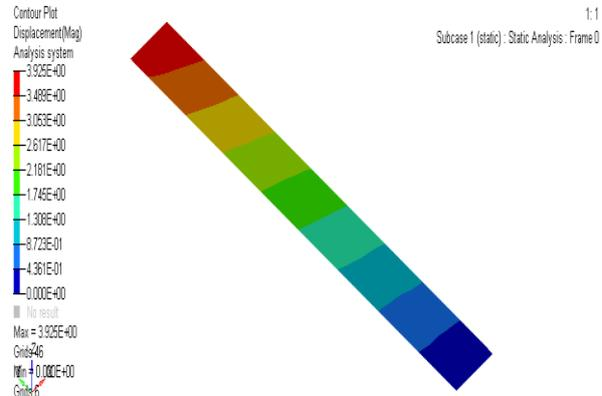
Fig. 28. Maximum displacement in the Y direction for the S2 sample
