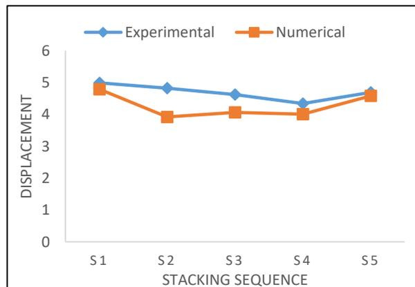
Fig. 37. Comparative study of displacement results with respect to stacking sequences.
