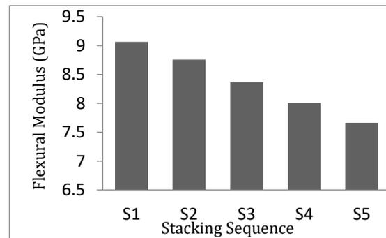
Fig. 24. Variation of specimen flexural modulus with reference to stacking patterns
