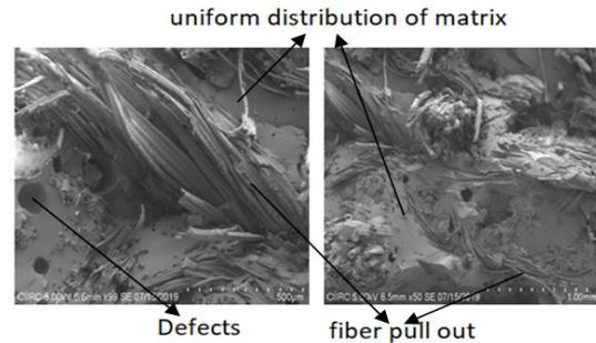
Fig. 54. Flexural test fractured SEM images of S1 Specimen (10% B and 20% J)
