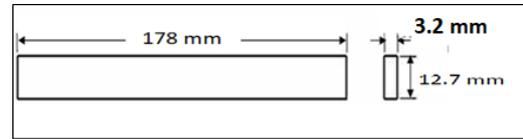
**Fig. 8.** Tensile Test Specimen dimensions
