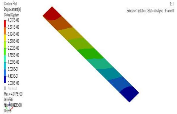
Fig. 32. Maximum displacement in the Y direction for the S4 sample
