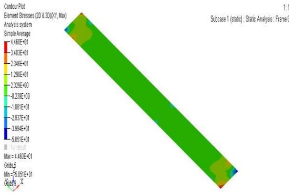
Fig. 25. Maximum stress in XY for the S1 Sample
