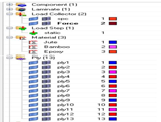
Fig. 16. Creating 13 plies for the stacking sequence S1
