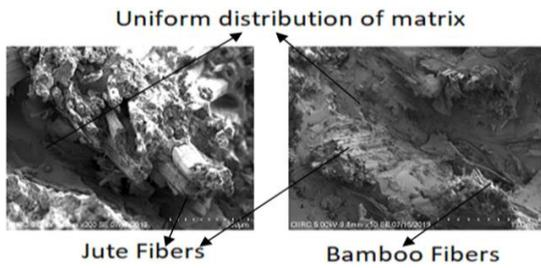
Fig. 38. Tensile test fractured SEM images of S1 specimen (10% B and 20% J)
