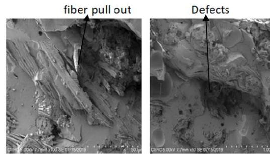
Fig. 55. Flexural test fractured SEM images of S2 Specimen (15% B and 15% J)
