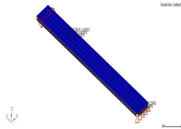
Fig. 17. Applying all the boundary conditions
