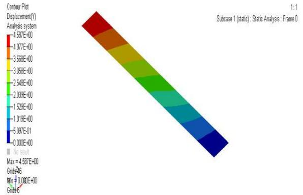
Fig. 34. Maximum displacement in the Y direction for the S5 sample
