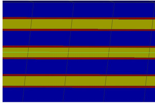
Fig. 15. Creating 13 plies for the S1 Stacking sequence
