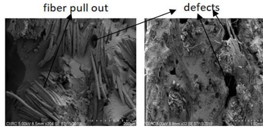
Fig. 40. Tensile test fractured SEM images of S3 specimen (20% B and 10% J)
