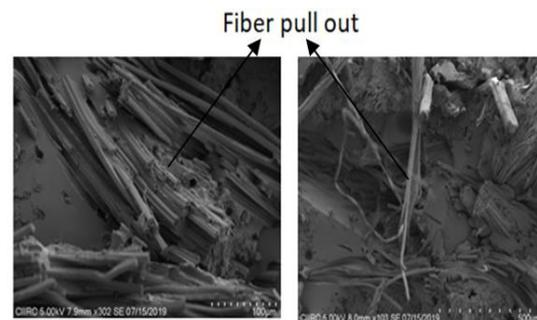
Fig. 56. Flexural test fractured SEM images of S3 Specimen (20% B and 10% J)
