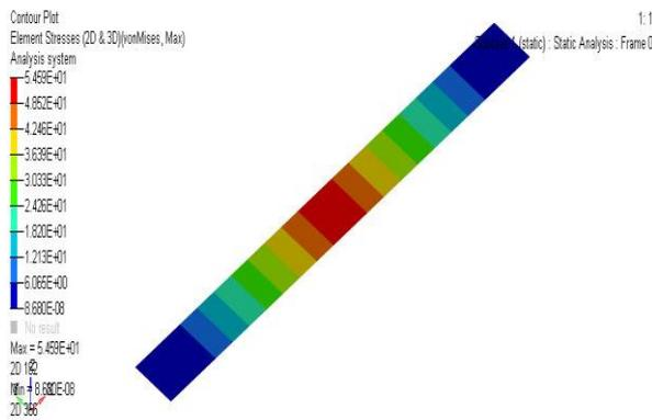
Fig. 47. Maximum von Mises stress for the S4 Sample
