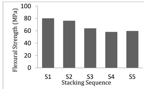
Fig. 23. Flexural strength of specimens varies according to the stacking order.
