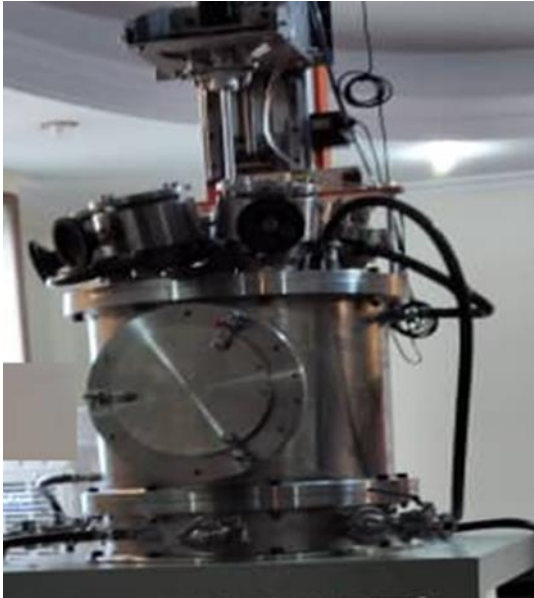
Fig. 2. Home-made Czochralski crystal growth system
