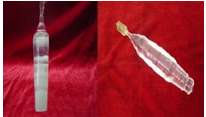
Fig.3. KCl crystals grown with 1.0 (left) and 0.5 (right) mole % Zn impurities.
