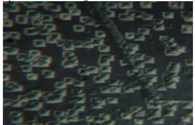
Fig.4. The etch-pits in the cleavage plane of KCl (Zn) crystals grown with 0.5 mole % impurity.
