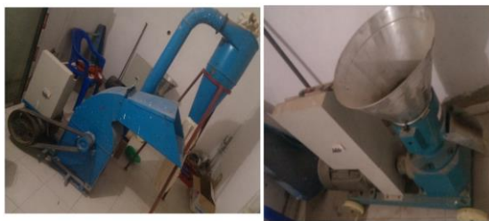
Fig. 2. Pictures of the hammer mill and pellet machine
