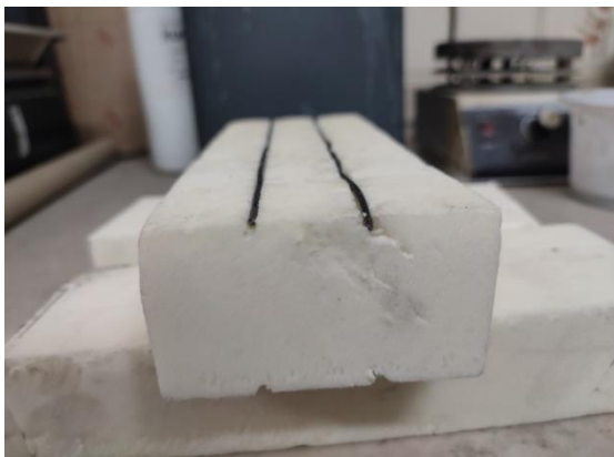
Fig. 2. Wire placement into the foam core
