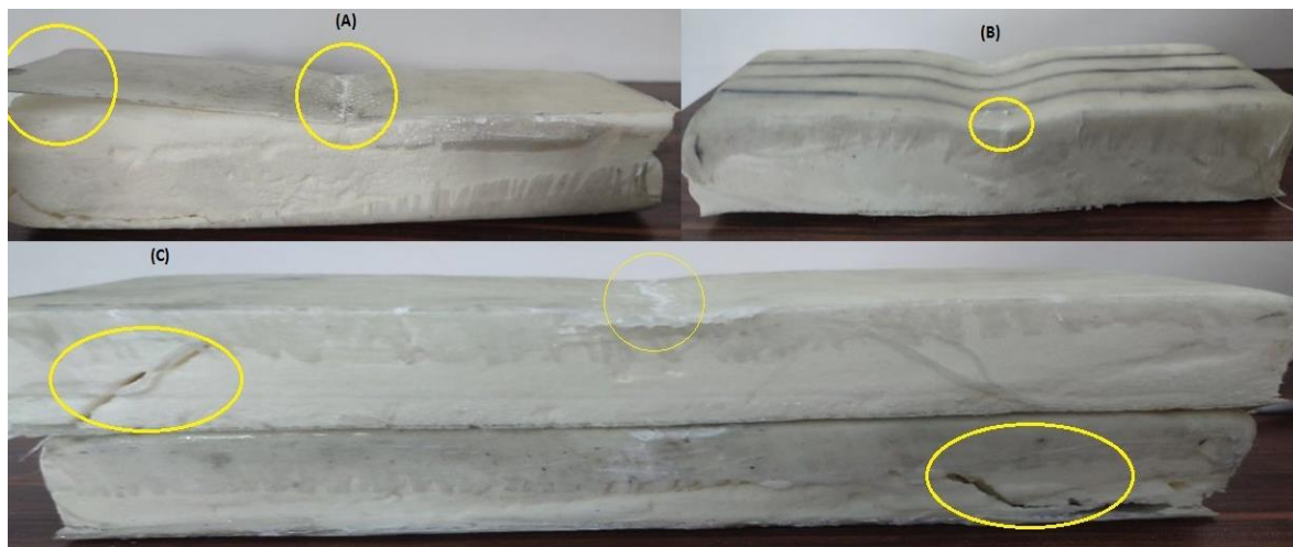
Fig. 11. Failure and damage mechanism of the sandwich structure subjected to three-point bending test A&C) NS panels and B) RS3 panel
