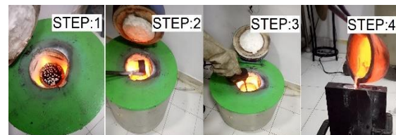
Fig. 4. Stir casting setup and pouring of Al6082 / AlSi10Mg molten metal into a die
