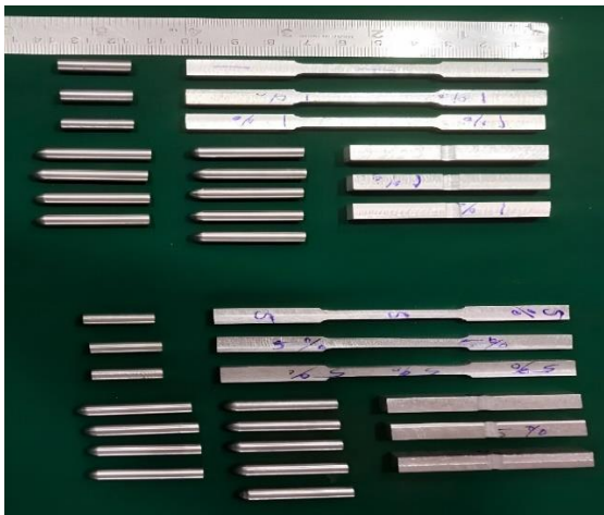
Fig. 6. Test samples of stir-casted Al6082 / AlSi10Mg composition
