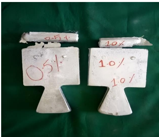
Fig. 5. Stir cast Al6082 / AlSi10Mg unmachined material
