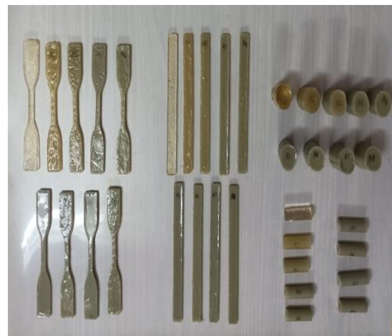
Fig. 1. Pictures of the fabricated samples for conducting various tests.
