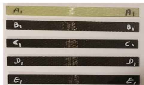
Fig. 12. Failed samples after Flexural test
