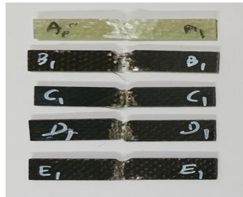
Fig. 15. Failed samples after Impact test
