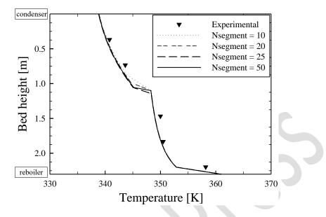
Fig. 5. The predicted temperature profiles along the packed height based on several segment size
