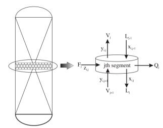
Fig. 1. Schematic representation of a segment in the packed column
