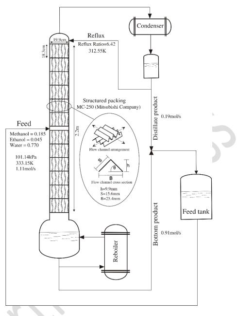
Fig. 4. Schematic representation of the packed distillation column in addition to packing specifications
