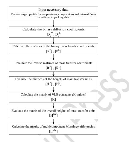
Fig. 2. The sequence of multicomponent efficiency calculations for each segment
