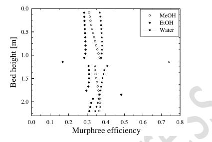
Fig. 7. Calculated efficiencies for different components as a function of the packing height
