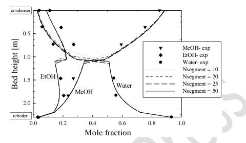
Fig. 6. Liquid mole fraction profiles of all components along the packed height for different segment size
