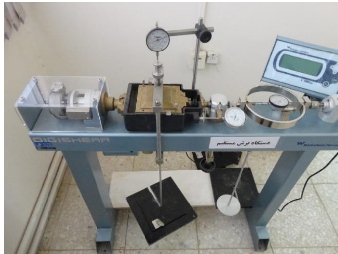
Fig. 4. Direct shear apparatus used in experimental program.
