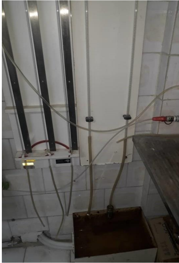
Fig. 5. Permeability apparatus used in experimental program.
