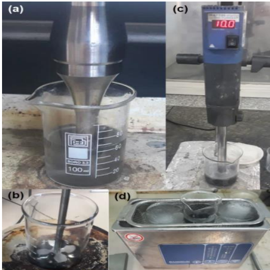
Fig. 7. A view of (a) ultrasonic probe; (b) mechanical mixing; (c) high shear turbo mixer; (d) ultrasonic cleaner.
