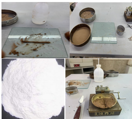
Figure 4: Performing a flow limit and plastic limit test
