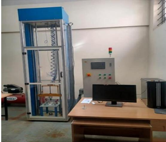
Fig. 2. Low-velocity impact testing machine
