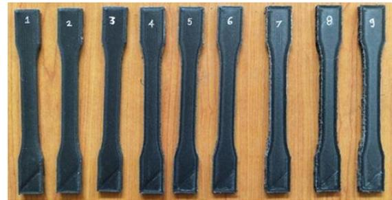
Fig. 4a. Tensile strength sample ASTM D 638 standard
