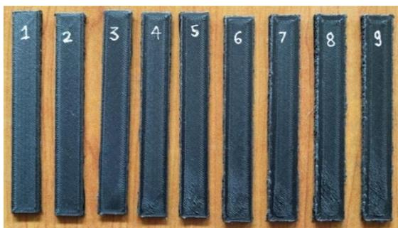
Fig. 3a. Flexural-test-specimen-as-per-ASTM-D790
