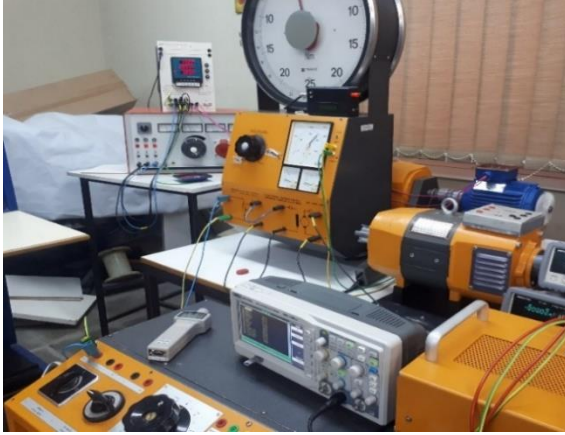
Fig. 3. Laboratory set to calculate the rotor bars' current
