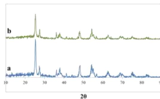
**Fig. 3.** XRD patterns of a) n-TiO<sub>2</sub>-P25, and b) Henna sensitized n-TiO<sub>2</sub>-P25.
