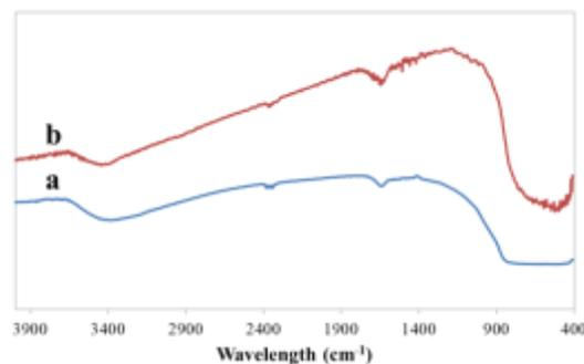
**Fig. 2.** The FT-IR spectra of a) bare n-TiO<sub>2</sub>-P25 and b) henna sensitized n-TiO<sub>2</sub>-P25.
