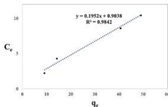
Fig. 8. Equilibrium data on the adsorption of henna dye on n-TiO<sub>2</sub>-P25 particles.
