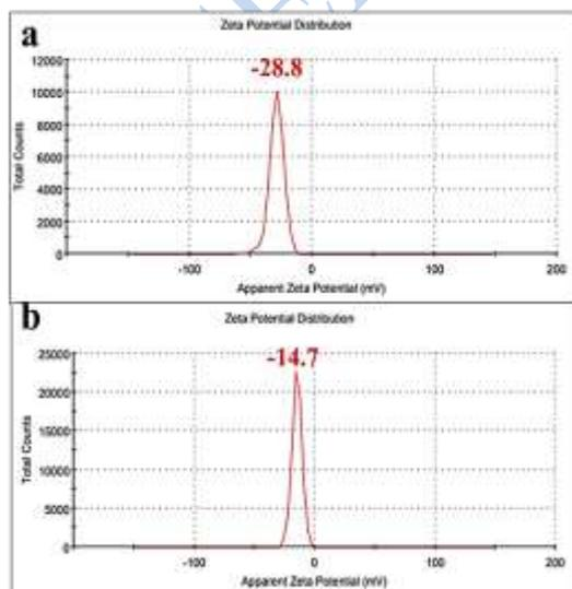
**Fig. 9.** Zeta potential determination of a) bare n-TiO<sub>2</sub>-P25 and b) henna sensitized n-TiO<sub>2</sub>-P25.
