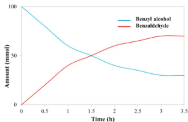
**Fig. 12.** Experimental results of oxidation of benzyl alcohol by henna sensitized n-TiO<sub>2</sub>-P25 under blue light irradiation.
