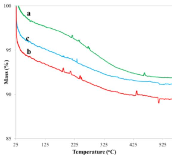
**Fig. 1.** TGA curves of n-TiO<sub>2</sub>-P25 sensitized with a) 1mg/L, b) 3mg/L, and c) 5mg/L henna.
