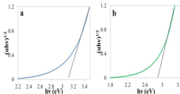
**Fig. 11.** Kubelka–Munk energy curve plots of a) bare n-TiO<sub>2</sub>-P25 and b) henna sensitized n-TiO<sub>2</sub>-P25.
