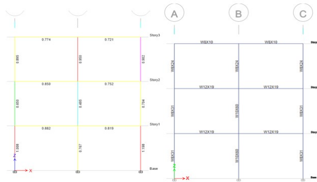
Figure 21: Stress ratio in a 3-story structure using the Etabs- (W section) ASD
