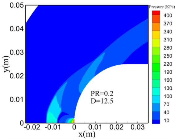
d) Jet Injection with Pressure Ratio 0.2
