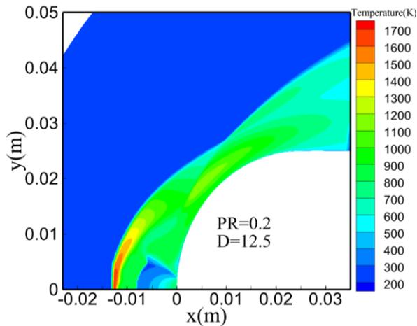
d) Jet Injection with Pressure Ratio 0.2
