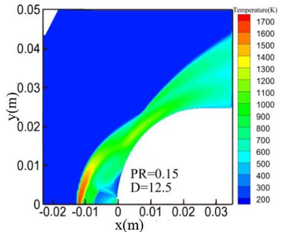
c) Jet Injection with Pressure Ratio 0.15
