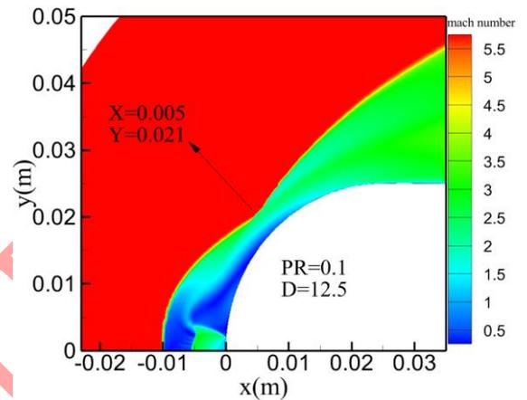
51 b) Jet Injection with Pressure Ratio 0.1
