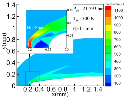
6 **Fig. 23.** Static Temperature Contour in Double Cone Geometry
