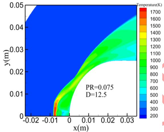
a) Jet Injection with Pressure Ratio 0.075
