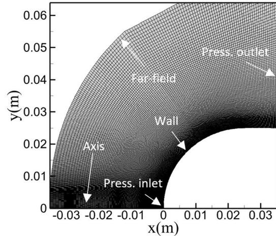
Fig. 2. Structured Mesh of the Computational Domain
