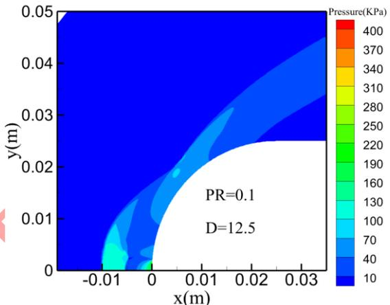
b) Jet Injection with Pressure Ratio 0.1
