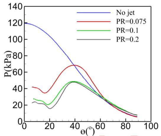
Fig. 8. Pressure Distribution on the Surface of the Geometry at Various Jet Injection Pressure Ratios
