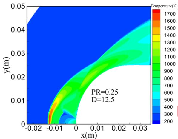
e) Jet Injection with Pressure Ratio 0.25
