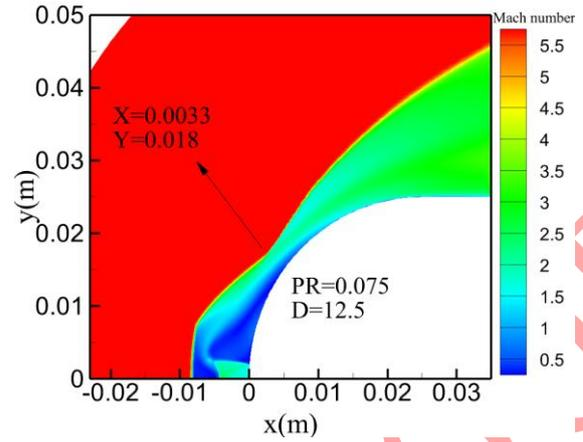
50 a) Jet Injection with Pressure Ratio 0.075
