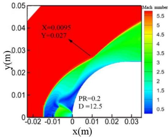
d) Jet Injection with Pressure Ratio 0.2
