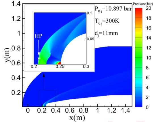
a) Static Pressure Contour at 10.897 Bar Jet Injection Pressure
