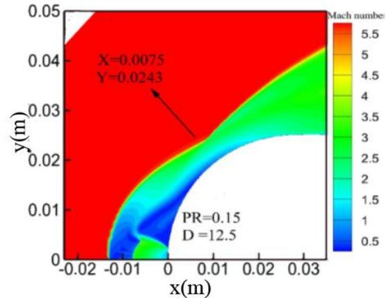
52 c) Jet Injection with Pressure Ratio 0.15
