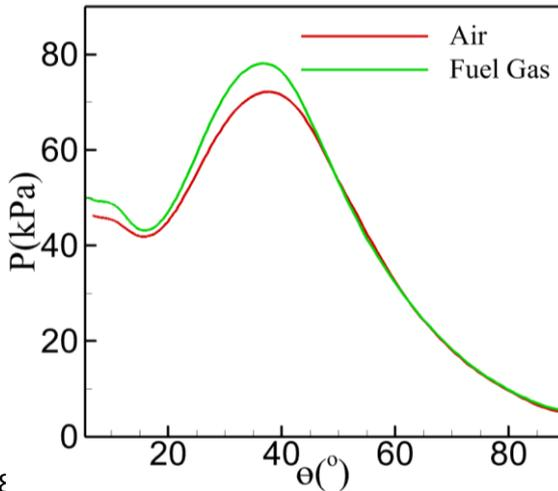
9 a) Pressure Distribution on the Surface of the Nose
