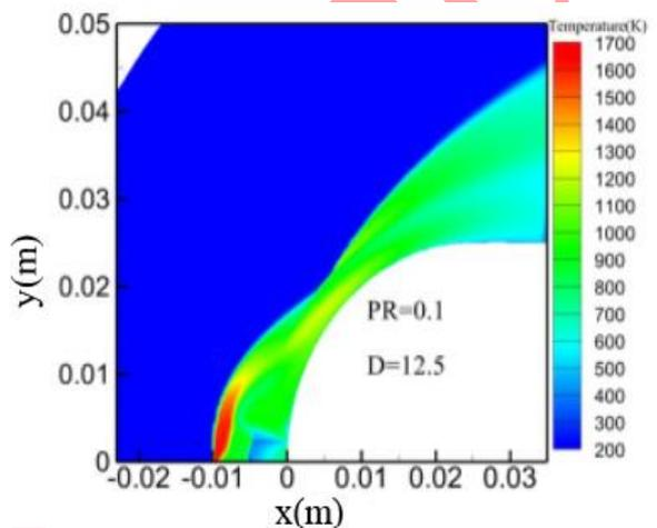
b) Jet Injection with Pressure Ratio 0.1
