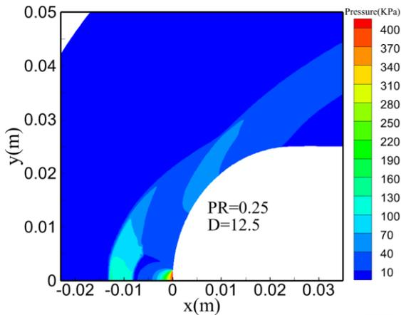
e) Jet Injection with Pressure Ratio 0.25
