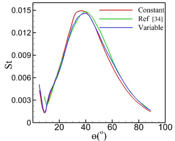
Fig. 4. Variations of the Stanton Number on the Nose as a Function of the Angle  $\theta$  for Constant and Temperature-Dependent Values
