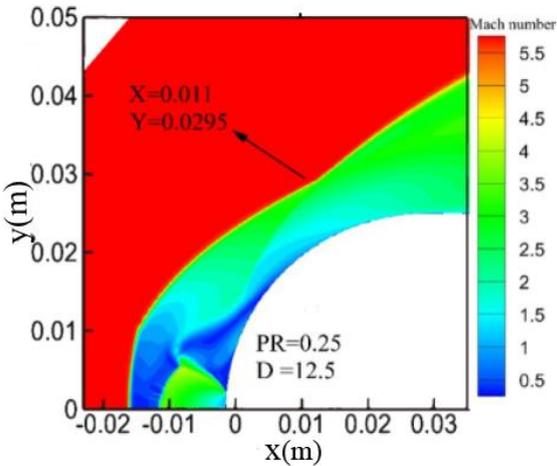
e) Jet Injection with Pressure Ratio 0.25
