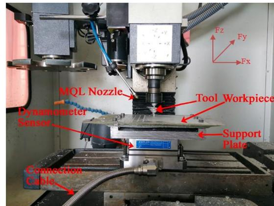
**Fig. 2.** The Machining Setup
