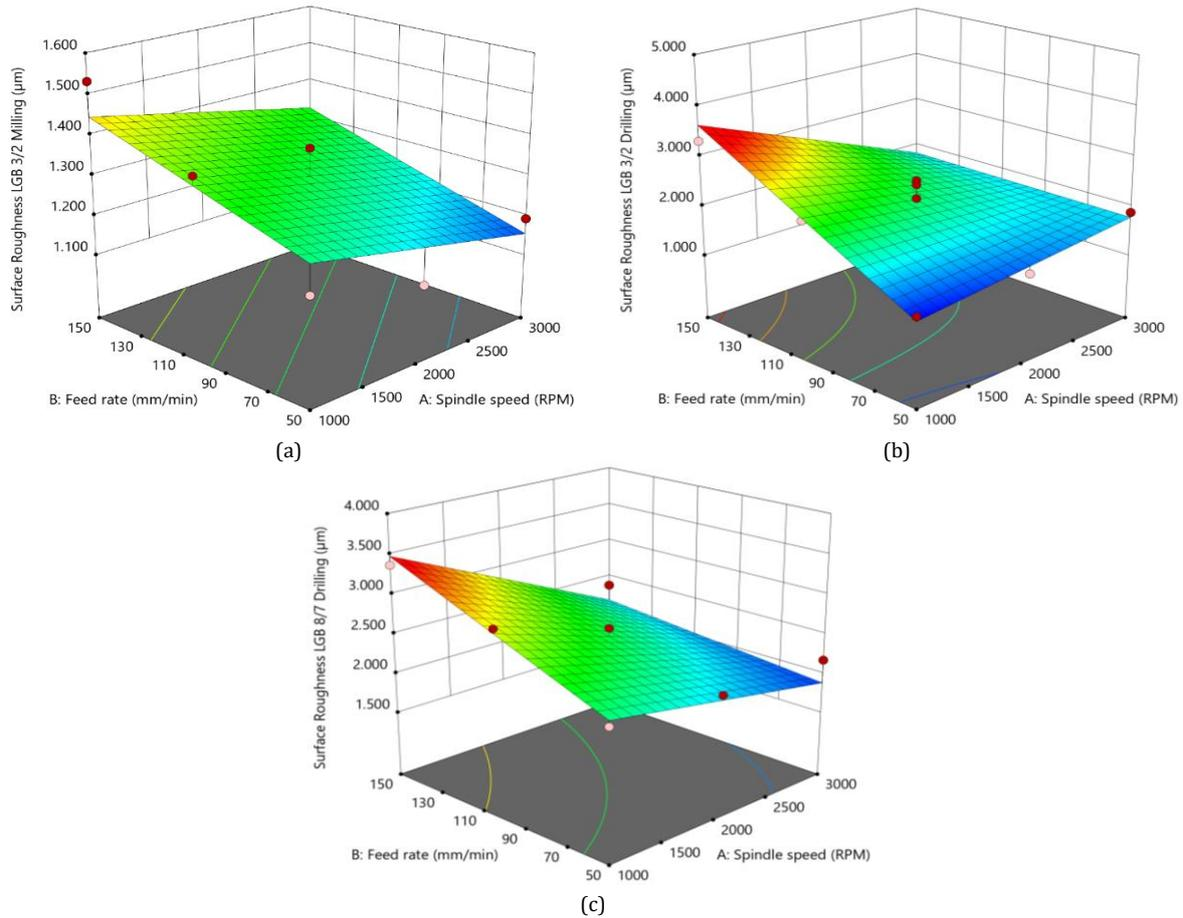
Fig. 9. 3D Response Contour Plot Showing the Interaction Between Spindle Speed and Feed Rate on Surface Roughness Under MQL Conditions: (a) Helical Milling with LGB3/2, (b) Twist Drilling with LGB3/2, (c) Twist Drilling with LGB8/7
