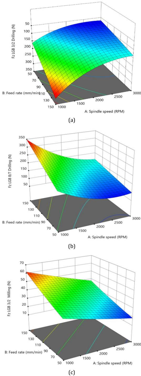
**Fig. 5.** 3D Response Contour Plot Showing the Interaction Between Spindle Speed and Feed Rate on Thrust Force (Fz) Under Dry Conditions: (a) Twist Drilling with LGB3/2, (b) Twist Drilling with LGB8/7, (c) Helical Milling with LGB3/2
