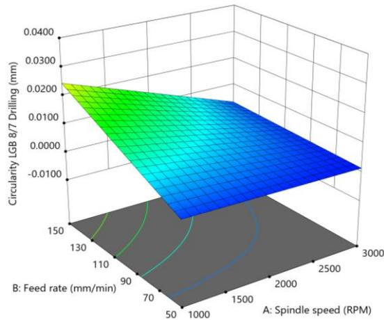
**Fig. 11.** 3D Response Contour Plot Illustrating the Interaction Between Spindle Speed and Feed Rate
