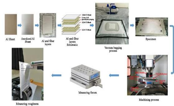
Fig. 3. Schematic Representation of the Process Steps
