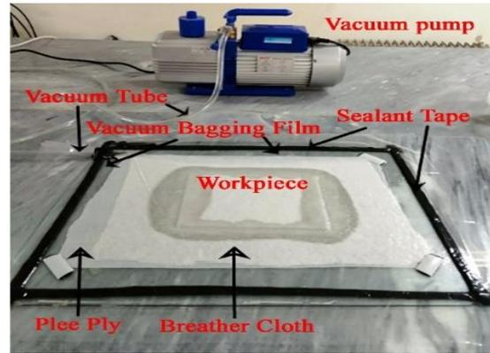
**Fig. 1.** Hand Lay-Up Method and the Use of the Vacuum Bagging Process
