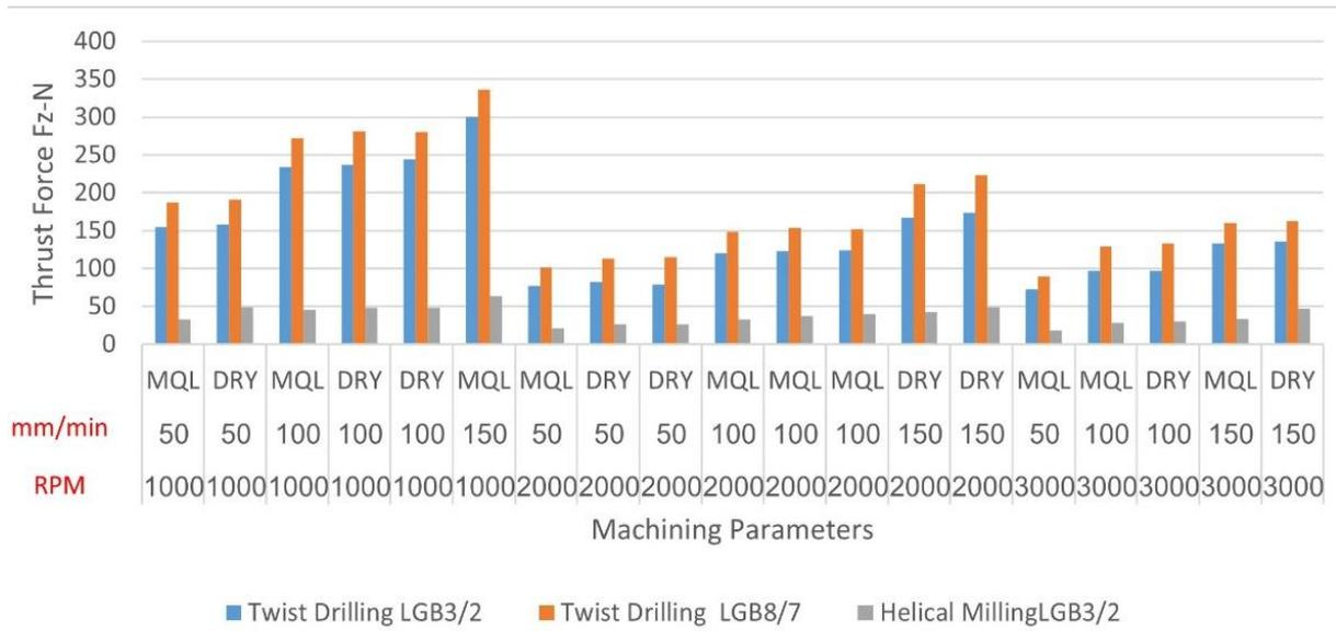
Fig. 4. Thrust Forces and Their Variations Due to Different Processes and Machining Parameters
