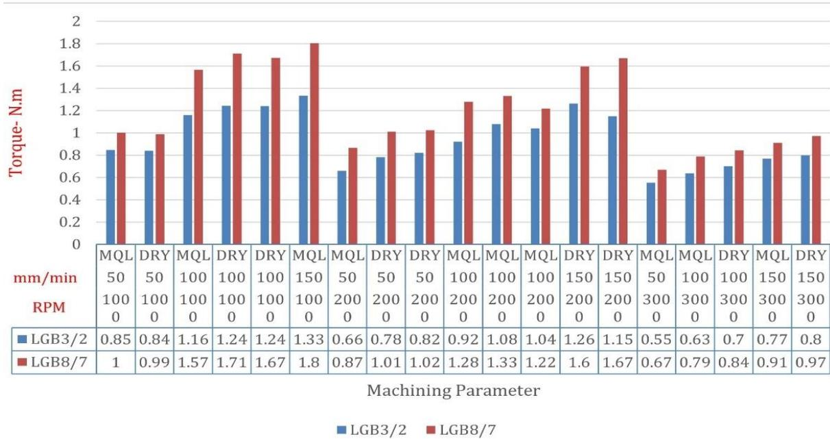
Fig. 6. Variations in Torque During Twist Drilling Based on Machining Parameters
