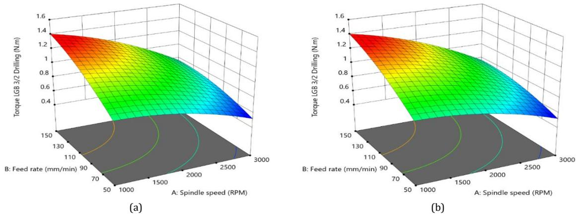
Fig. 7. 3D Response Contour Plot Illustrating the Interaction Between Spindle Speed and Feed Rate on Torque under Dry Conditions: (a) Twist Drilling with LGB3/2, (b) Twist Drilling with LGB8/7
